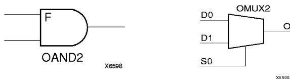
Figure 20: AND & MUX Symbols in XC4000X IOB
